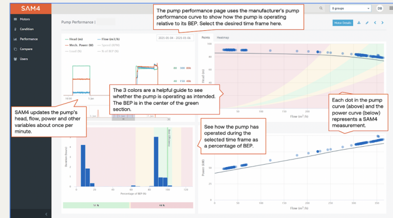
(a) sample real-time pump curve and performance metrics
