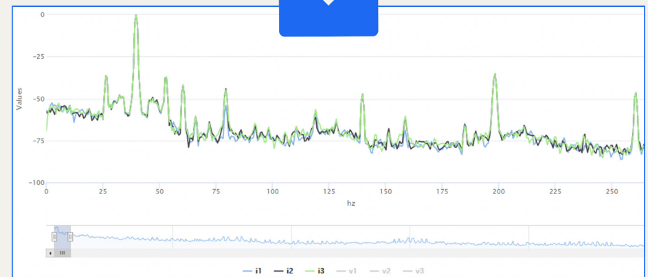
Figure 6. Every motor and machine has a different healthy pattern, which the condition monitoring system must learn if it's going to detect developing faults early enough to help. Recent advances in machine learning have brought this level of detection within reach.
